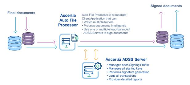
AFP is an intelligent Java application using ADSS Client SDK to handle interactions with ADSS Server. It is controlled by an XML configuration file that defines which folders to monitor, which file types to look for, which ADSS Servers to communicate with, how to handle issues that might arise and more.
