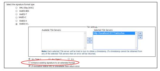
The grace period field is a very useful element for those projects that require this capability. In addition if revocation information is not available, e.g. a back-end OCSP responder fails to reply, then a setting enables the signing operation to fail and return an error condition. This is vital as many other products simply do not enforce such policies and "assume" its okay to continue without this information. It will be expensive and awkward to discover this sometime later!
