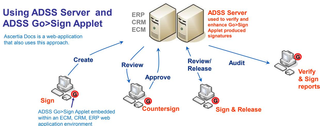
The core signing functionality is within Go>Sign Applet and the policy controls reside within the application or alternatively within ADSS Server. The ADSS Server security management interface ensures that only role-privileged operators can change these policies and if required dual controls can be enabled so that 'four-eyes' control can easily be applied.
