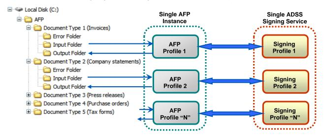
The diagram illustrates multiple AFP profiles processing various document types located in different input folders. The documents are then signed on the ADSS Server using unique signing profiles and the resultant file deposited in the appropriate output folder.
