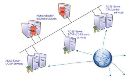
adapted to suit changing loading conditions using the in-built flexibility of the product. Additional servers can be utilised to run more OCSP services and thus handle greater loads. Similarly SCVP, XKMS and even DSS verification services can be added as needed on the same or different production servers. All verification
